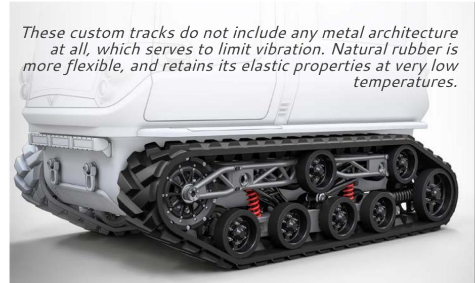
*These custom tracks do not include any metal architecture at all, which serves to limit vibration. Natural rubber is more flexible, and retains its elastic properties at very low temperatures.*
