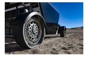
From 2026, when the FLEX rover is put into service at the lunar south pole, where extreme temperatures (-90 to -230°C) prevail, the four wheels supporting the two-tonne vehicle (payload included) will warp in order to absorb ground irregularities as
